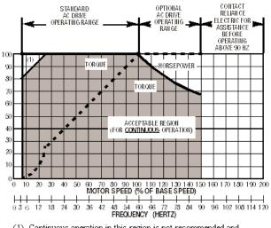
Continuous operation in this region is not recommended and may result in reduced motor life.
