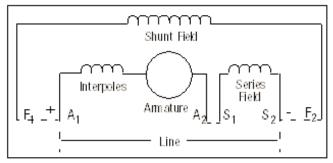
Stabilized shunt motors utilize a field winding in series with the armature in addition to the shunt field to obtain a compromise in performance between a series and shunt type motor. This type offers a combination of good starting torque and feed stability.
