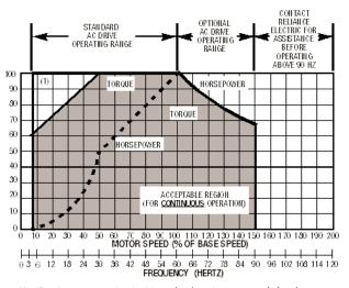
Continuous operation in this region is not recommended and may result in reduced motor life.
