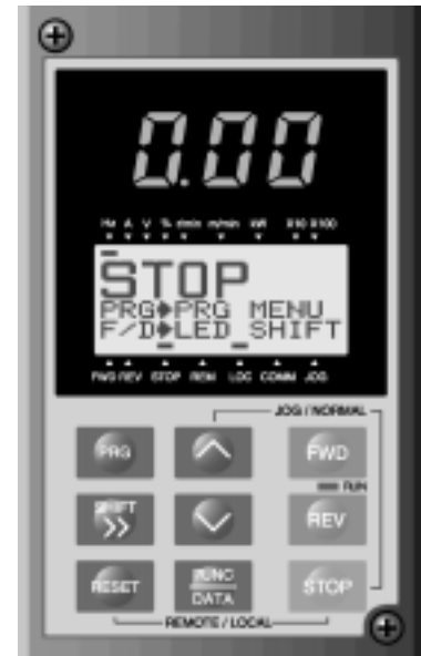
Fig. 3-1-2 Display on keypad panel at power-on
